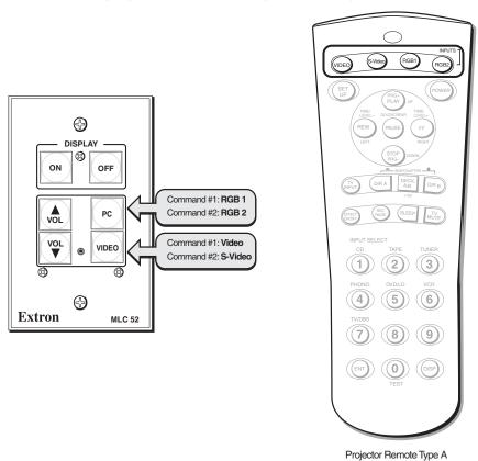
Programming MLC 52 input selection buttons from a projector remote control type A
